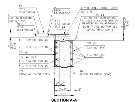
DECK SLAB SHOWN FOR INFORMATIONAL PURPOSES ONLY DO NOT PLACE DECK SLAB CONCRETE UNTIL THE ABUTMENT DIAPHRAGM CONCRETE HAS ATTAINED A COMPRESSIVE STRENGTH OF 3000 P.S.I.
